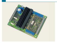
The electronic control Unit ES/43 is designed for controlling proportional valves without position control.
