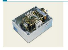
The gearing limit switch GE1 is a rugged switching device in accordance with IEC 947-5-1 EN 60947 DIN VDE 0660-200 designed for hoisting applications. The modular micro changeover contacts have positive openings.
