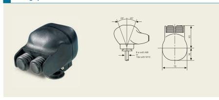
The palmgrip B2 is an actuating element for the multi-axis controllers V8. It can also be used as an actuating element for hydraulic drives. With each of the two pushbutton one direction-contact (micro changeover contact) also one potentiometer pushed. These palmgrips enable the 3 direction 9-10 (3. axis) on the multi-axis controller V8.
